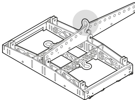
Use of the frame and suspension bar with a single central lifting point. Recommended for an array configuration of up to 16 MYRA 214L modules.
