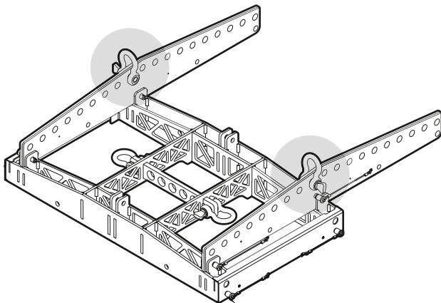
Using two side suspension bars and two lifting points. Recommended for an array configuration of 16 to 24 MYRA 214L modules.
