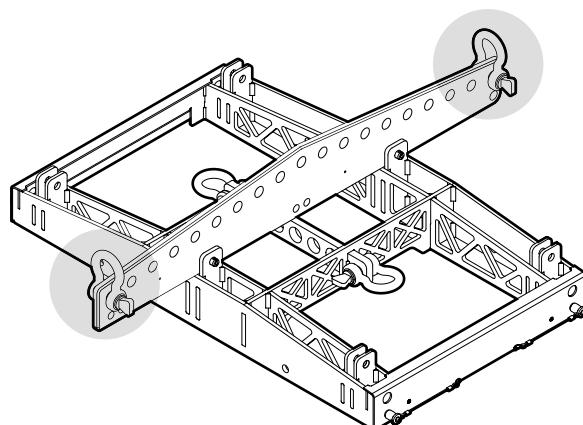
Use of the suspension bar in a central position with two lifting points; this configuration provides the best weight distribution. Recommended for an array configuration of 16 to 24 MYRA 214L modules.
