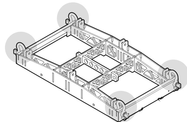
Use of the frame only, without the suspension bar and with four lifting points. Recommended for an array configuration of up to 24 MYRA 214L modules in fixed and permanent installations.
