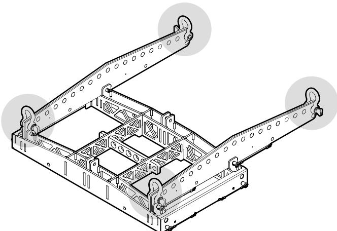
Using two side suspension bars and four lifting points. Recommended for an array configuration of 16 to 24 MYRA 214L modules.
